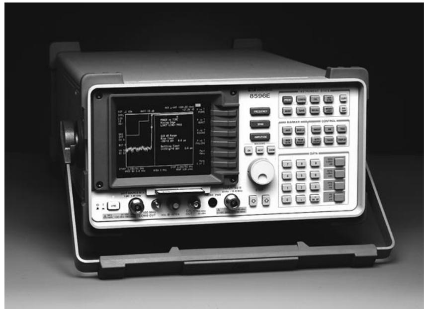
The HP 8590E options 012 and 112 complete the spectrum analyzer solution for your DECT transceiver testing needs. The option 112 DECT demodulator card, gives the capability to analyze the modulation on the transmitted DECT signals and display the demodulated data in real time on the spectrum analyzer screen.
